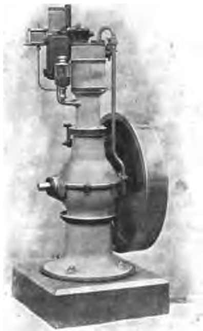
FIG. 288. —A Daimler Single-Cylinder Motor Intended for Stationary Use. Attached to the head of the water-cooled cylinder are the gasoline chamber and carburetter. The lubricating cup is shown immediately below. The exhaust valve, not shown, is operated by a cam on the secondary shaft, geared to the crank shaft, as may be seen within the fly-wheel. In essential particulars this motor is identical with those used for vehicle propulsion; the method of mounting being, of course, different.
